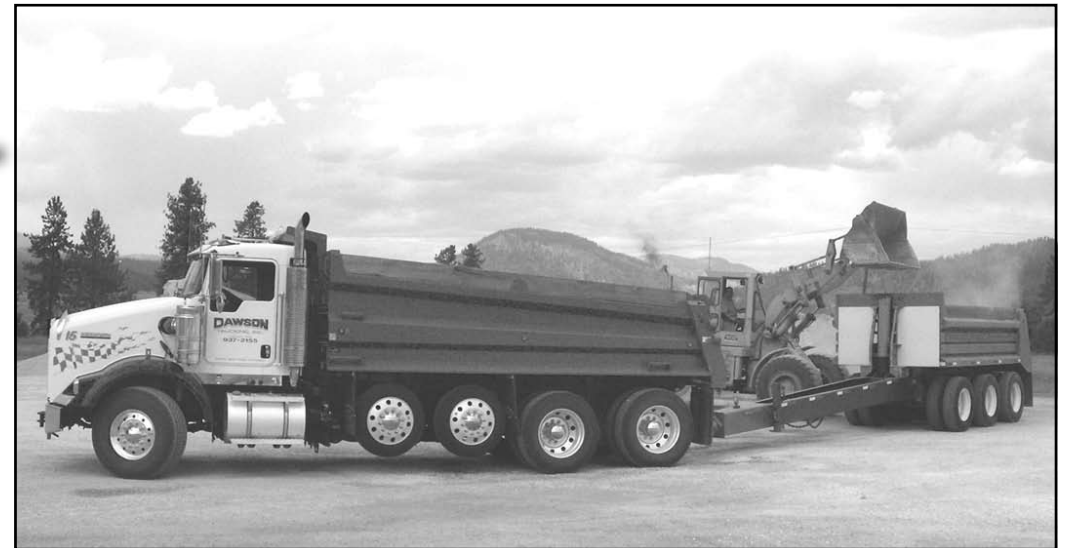
A Dawson Trucking gravel truck and pup get loaded up to haul out and deliver. Photo Huckleberry Press.
